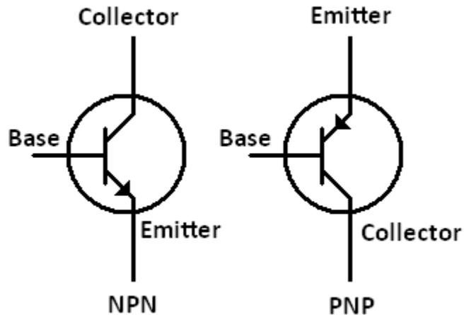
Figure 2.: Transistor Notations
