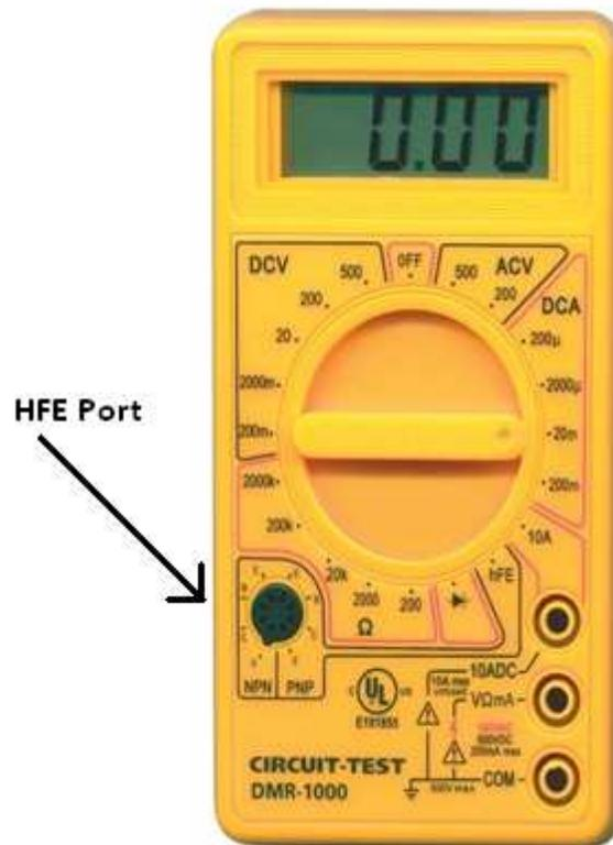
Figure 4.: HFE port on multimeter
